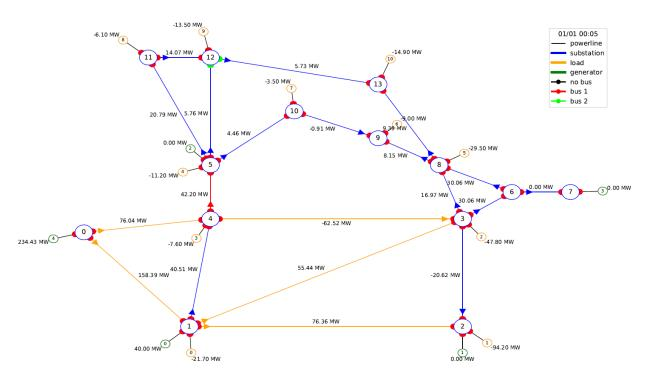
• The topology surrounded in orange has got a 1 simulated score. It does resolved the power flow on line 9 but created an other one on an other line
