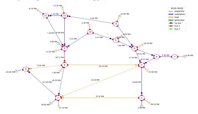
The simulator will then compute several objects to provide to AlphaDeesp, which will run a greedy algorithm to determine the best topological action to solve the overload. For more details, see the section *Algorithm Details*
